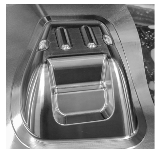
Excellent surface finish of 0.4 \mu\text{m} with SolidCAM HSM strategies
