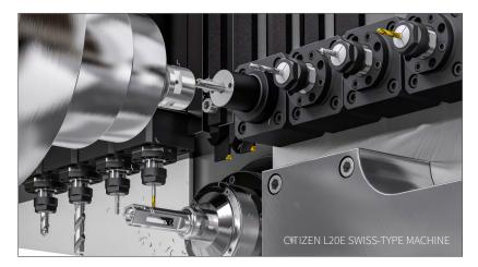
Parts are typically small, complex and often have high precision requirements. Swiss-Type Machines have a sliding headstock and a guide bushing through which the stock is fed, supported and nearby later cut. Such machines can also have a large number of axes, are exceptionally stable and regularly provide remarkable machining cycles.
